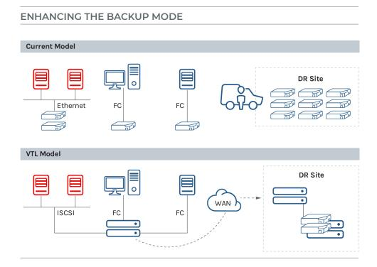
One of the bottlenecks of physical tape backup is the fixed number of tape drives. Once all drives are in use, backup streams/jobs begin to queue creating a bottleneck and slowing the overall backup process. The only solution is to add more physical drives or libraries, or to resort to tape-drive sharing, which can be complex to implement, can impact performance, and can require additional licensing fees.
