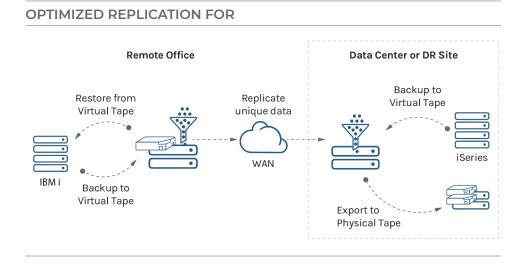
By using FalconStor VTL with IBM i, smaller offices and remote sites can electronically vault tapes across any distance using standard IP (WAN) networks, centralizing data at the DR site for long-term data protection, retention, and central tape creation. Data over the wire is encrypted (AES 256-bit) and data written from the FalconStor VTL directly to physical tape can also be encrypted (AES 256-bit), ensuring data is safe at all times.
